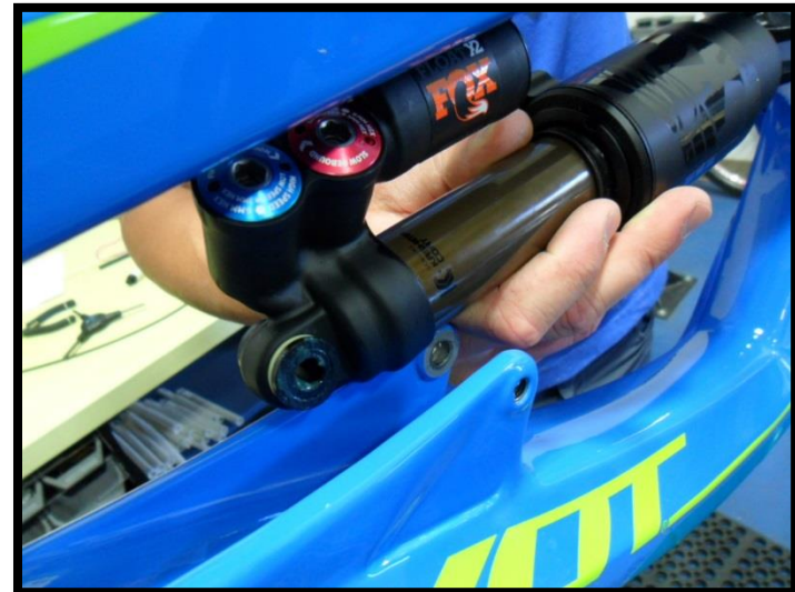
Step 6. Install front of shock over shock tabs.
