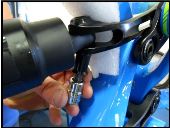
Step 5. Install clevis shock bolt first.
